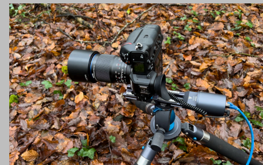
CASTEL-MICRO electronic rail in with the MagicBall. Ideal for automatic focus bracketing.
