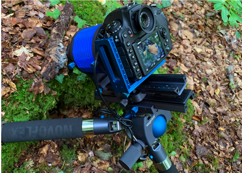
The MagicBall is more than capable of supporting setups such as this double rail configuration with the BALPRO-1 bellows and the vintage Novoflex 60mm flat field macro for higher reproduction imagery:
