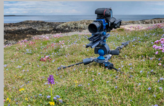
BAL-F bellows, Schneider Kreuznach Pyrite F4.5/90mm and the CASTEL XQ II focusing rail.
