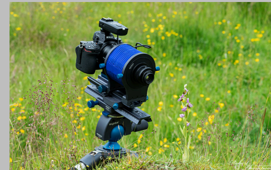
BALPRO 1 bellows, Nikon 50mm EL lens and the CASTEL XQ II focusing rail.
