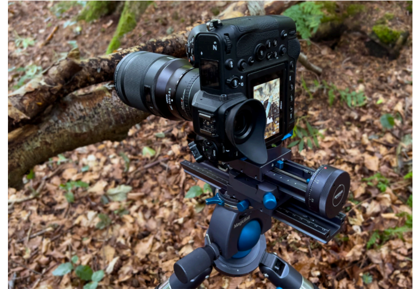
The Castel-M and CASTEL XQII focusing rail for precise placing of the focusing point. The additional rail is useful when working at magnifications beyond 1:1 and saves time repositioning the tripod.
